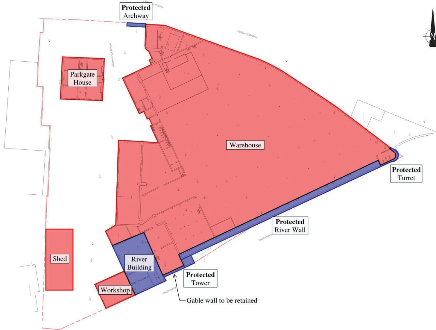
Figure 4.2: Layout of existing structures (red reflects demolition; blue reflects to be retained)
